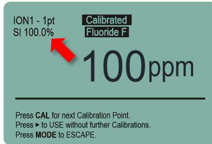
The instrument is now calibrated. The slope will be indicated and be 100%.
