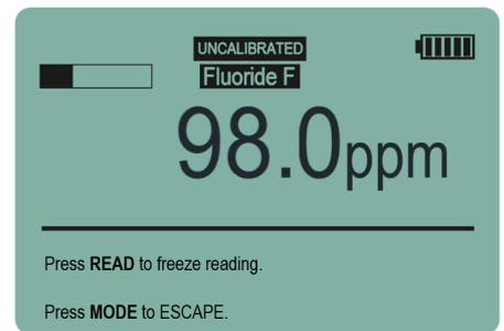
Insert the ISE into the standard and press **READ**.
