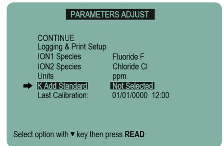
Press the **down arrow** and select the 'K Add Standard' tab and press **READ**.
