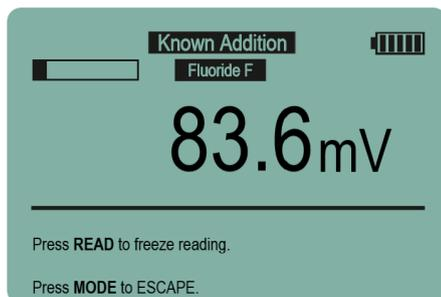
Add 10ml of the standard solution to the same beaker, stir and press **READ**.
