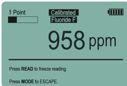
Then insert the ISE into the standard and press **READ**.
