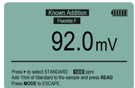
Press the **right arrow** to select the standard you are using and press **READ**.
