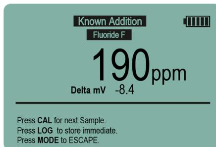
The QP459 will measure the solution and display the result, when stable, in direct concentration units.
