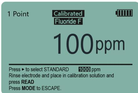
For a 2-point calibration press **CAL** and then select the second standard.
