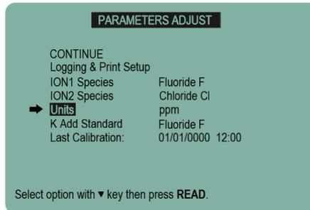
Press the **down arrow** to select 'Units' and press **READ** to select ppm or mol/l
