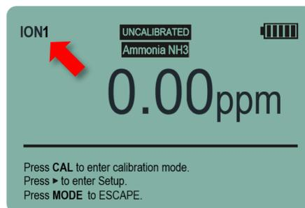
Press **MODE** until ION1 is displayed in the top-left hand corner of the display.
