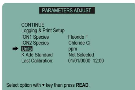
Press the **down arrow** to select 'Units' and press **READ** to select either ppm or mol/l.
