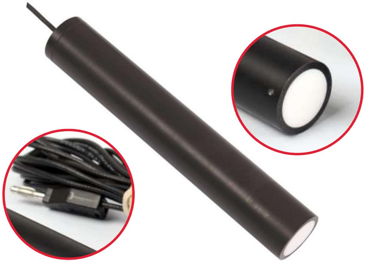
The Cathodic Protection Reference Electrode from EDT directION is a Silver /Silver Chloride Reference electrode designed to enable the measurement of the condition of boats and submerged metal structures in both Freshwater and Saltwater applications.
