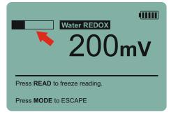
The **stability bar** will fill up and the reading will freeze once the measurement is stable.
