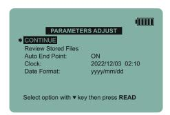
Press **right arrow** after unfreezing the display. This takes you to the "**PARAMETERS ADJUST**" screen.
