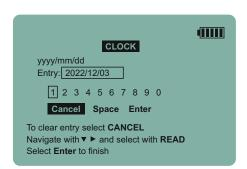
Select **CANCEL** using the down arrow key and press **READ** until the current **DATE** in the entry box is removed.
