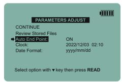
From the **PARAMETERS ADJUST** screen select Auto end Point Now press **READ** to switch on Auto End Point.
