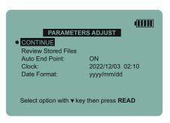
Press the **right arrow** key to enter the PARAMETERS ADJUST SCREEN
