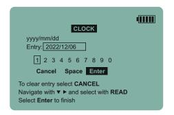
When the entry box contains the correct date select **ENTER** and press **READ**
